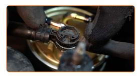
18 Install the fuel filter pipe retainer.
