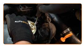
Remove the o-rings. Use a flat screwdriver.
