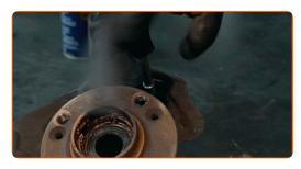
Remove the brake disc cover.
