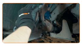
Attach the ball joint to the control arm. Use a pin punch.
