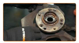
Screw in the fasteners of the brake disc cover. Use a drive socket #8. Use a torque wrench. Tighten it to 5 nm torque.
