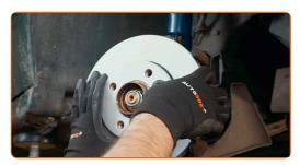
Tighten the brake disc fastening. Use Torx T27. Use a torque wrench. Tighten it to 9 Nm torque.
