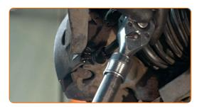
11 Remove the brake caliper.
