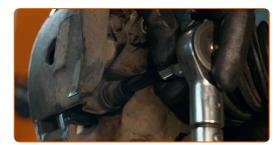
Treat the fasteners of the ball joint. Treat the CV axle fastener. Treat the fastener connecting the tie rod end to the steering knuckle. Treat the shock strut fasteners. Use copper grease.
