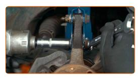
Remove the fastening bolt.
