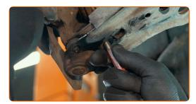
Screw in the fastener connecting the ball joint to the control arm. Use a drive socket #13. Use a ratchet wrench.
