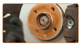
67 Clean the brake disk surface. Use a brake cleaner.
