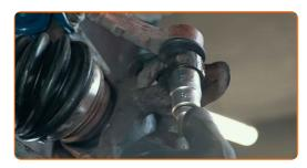
Tighten the fasteners connecting the ball joint to the control arm. Use a drive socket #13. Use a torque wrench. Tighten it to 20 Nm torque.+90°
