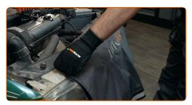
Unscrew the air filter housing fasteners. Use a Phillips screwdriver.
