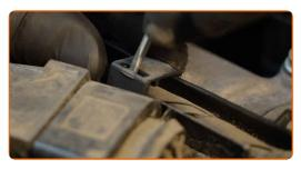
5 Detach the connector from the ignition coil.
