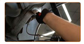
Install the rubber spacer on the new coil spring.
