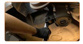
Remove the fastening bolt. Use a combination spanner #16. Use a drive socket #16. Use a ratchet wrench.
