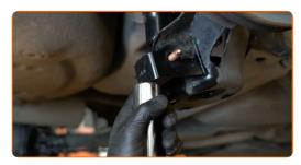
Screw in the lower fastener of the shock absorber. Use a combination spanner #16. Use a drive socket #16. Use a ratchet wrench.
