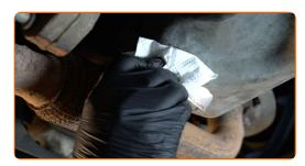
Screw in the new drainage plug and tighten it. Use a drive socket #19. Use a torque wrench. Tighten it to 26 Nm torque.
