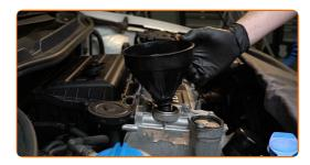
Pour oil into the engine through the filler. Required amount of oil: 3.6 l.
