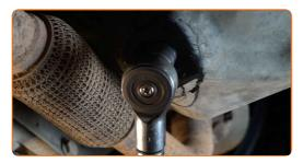
Clean the area of the oil pan drainage hole. Use all-purpose cleaning spray.
