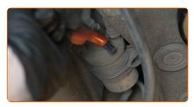
Disconnect the fuel supply lines from the fuel filter. Use a flat screwdriver. Use a crowbar.
