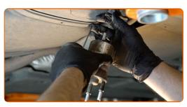
Connect the fuel supply lines to the fuel filter.
