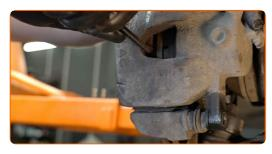
10 Remove the brake caliper.
