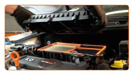
Remove the filter element from the filter housing.
