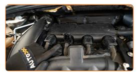
Detach the connector from the ignition coil.
