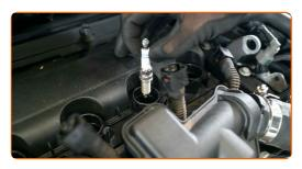
Screw new spark plugs and tighten them. Use the 12-point spark plug socket #14. Use a torque wrench. Tighten it to 23 nm torque.
