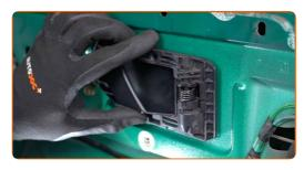
Lower the glass so that you can see the fasteners that connect it to the window regulator mechanism.
