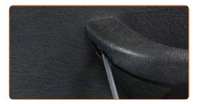
6 Unscrew the door handle fastener. Use Torx T30.
