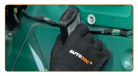
Tighten the fasteners of the window regulator assembly. Use a drive socket #10. Use a torque wrench. Tighten it to 12 Nm torque.
