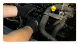
Attach the fuel pressure sensor connector.
