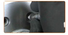
Tighten the brake drum fasteners. Use Torx T30. Use a torque wrench. Tighten it to 10 Nm torque.
