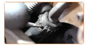
Remove the upper return spring of the brake shoes. Use a flat screwdriver.
