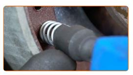
Install the brake shoe adjuster.
