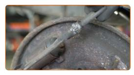
Remove the parking brake retaining spring of the left brake shoe. Use a flat screwdriver.
