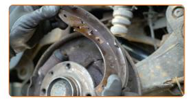
Remove the brake shoe adjuster.
