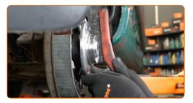
Treat the contacting surface. Use ceramic grease.
