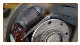
30 Install a new right brake shoe.
