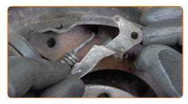
Loosen the brake shoe adjuster. Use a flat screwdriver.
