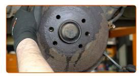
Clean the fasteners of the brake shoes. Use a wire brush. Use a brake cleaner.
