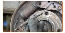
Remove the retainers of the drum brake shoes. Use a brake spring compressor tool.
