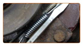
Install the parking brake retaining spring of the left brake shoe.
