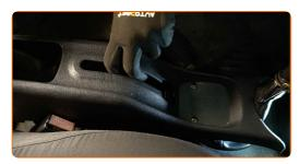
Loosen the parking brake cable adjustment nut. Use a drive socket #12. Use a ratchet wrench.
