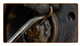
9 Remove the circlip.
