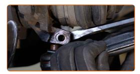
Disconnect the ball joint from the steering knuckle. Use a crowbar.
