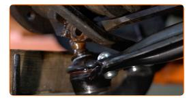
Unscrew the fastener connecting the drive shaft to the wheel hub.
