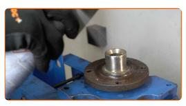
Install the wheel hub on the steering knuckle. Bush and bearing driver set.
