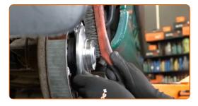
Treat the contacting surface. Use ceramic grease.
