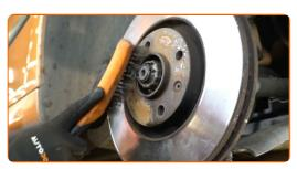
Unscrew the brake disc fastening. Use Torx T30. Use an impact screwdriver.
