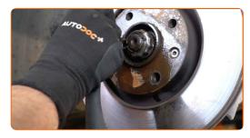
17 Remove the brake disc.
