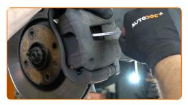
10 Remove the brake caliper.
