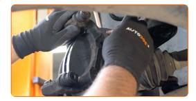
Tighten the brake caliper bracket. Use Torx T55. Use a torque wrench. Tighten it to 105 Nm torque.
