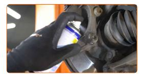
Unscrew the caliper bracket fastening. Use Torx T55. Use a tap wrench. Use a ratchet wrench.
