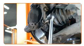
Remove the caliper bracket.
