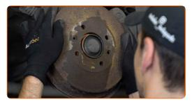
Tigten the brake drum fasteners. Use Torx T30. Use a torque wrench. Tighten it to 10 Nm torque.
