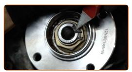
Apply special grease to the bearing assembly mounting seat. Use copper grease.
