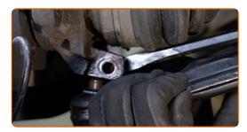
Disconnect the ball joint from the steering knuckle. Use a crowbar.
