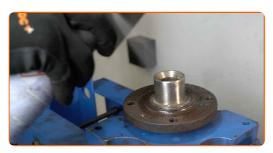
Install the wheel hub on the steering knuckle. Bush and bearing driver set.
