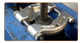
Press out the wheel hub bearing. Bush and bearing driver set.
