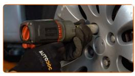
Lower the car and working in a cross order, tighten the wheel bolts. Use a torque wrench. Tighten it to 100 Nm torque.
