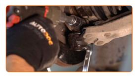
Remove the fastening bolt.
