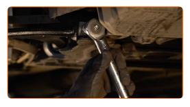
Remove the support from under the arm.
