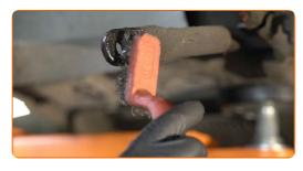
13 Install a new rod, tighten the fasteners.
