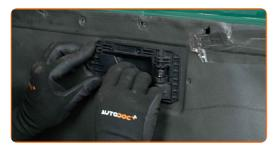
Reinstall the door card. Make sure you hear a click indicating that it is locked in place.
