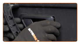
Screw in the lower fasteners of the door card. Use Torx T20.
