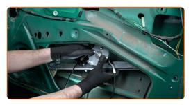
Treat the thread of the window regulator fasteners. Use threadlocker.
