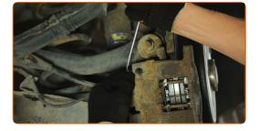
Unscrew the brake caliper fasteners. Use HEX No.H7.
