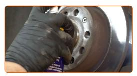
Unscrew the brake disc fasteners. Use Torx T30. Use a ratchet wrench.
