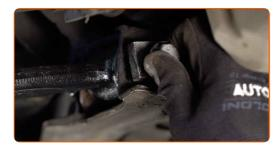
Screw the rear arm fastener. Use a combination spanner #13. Use a drive socket #16. Use a ratchet wrench.
