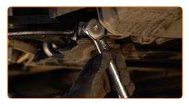
Remove the support from under the arm.
