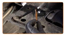
20 Install the front fastener of the arm.
