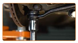
Tighten the front fastener connecting the control arm to the subframe. Use a drive socket #18. Use a torque wrench. Tighten it to 74 nm torque.
