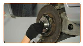
Tighten the hub. Use a drive socket #41. Use a torque wrench. Tighten it to 275 Nm torque.
