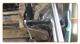
Tighten the top shock absorber fastening. Use a drive socket #24. Use a torque wrench. Tighten it to 110 Nm torque.
