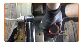
Remove the support from under the rear axle beam.
