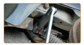
Unscrew the lower fastener of the shock absorber. Use a combination spanner #24. Use a drive socket #24. Use a ratchet wrench.
