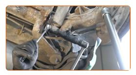
10 Remove the fastening bolt.
