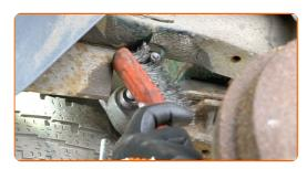
Treat the shock absorber mounting seats. Use copper grease.
