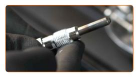
Install new glow plugs to their mounting seats. Use long nose pliers.
