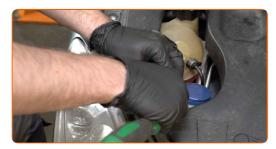
Remove the coolant reservoir cap.
