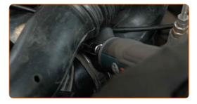
17 Remove the fender protection cover.
