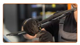
Remove the blade from the wiper arm.
