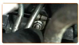
Tighten the fasteners that connect the power cables to the glow plugs. Use a drive socket #8. Use a torque wrench. Tighten it to 8 nm torque.
