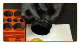
19 Install a new filter element into the oil filter cap.
