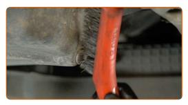
Unscrew the drain plug. Use a 13 mm socket. Use a ratchet wrench.
