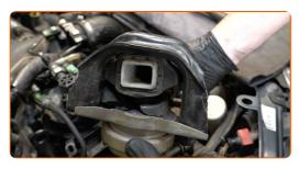
Replacement: engine mounts – PEUGEOT Expert Tepee (VF3X\_). AUTODOC recommends:
