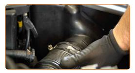
Tighten the binding clamps that attach the air duct to the air filter housing and to the charger. Use a combination spanner #7.
