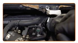
Tighten the clamp and fasteners on the air filter intake pipe. Use a combination spanner #7. Use a drive socket #10.
