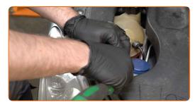
Remove the coolant reservoir cap.
