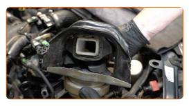
Replacement: engine mounts – PEUGEOT EXPERT Box (VF3A\_, VF3U\_, VF3X\_).
