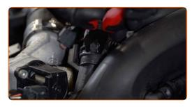
Unscrew the oil filler plug. Insert the funnel. 35
