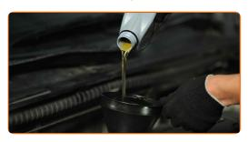
Replacement: engine oil and filter – PEUGEOT BOXER Platform/Chassis (244). Tip from AUTODOC experts:
