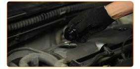
Tighten the oil filler cap.
