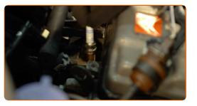
Screw new spark plugs and tighten them. Use the spark plug socket #16. Use a torque wrench. Tighten it to 28 nm torque.
