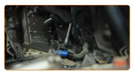
Plug in the ignition coil connector.
