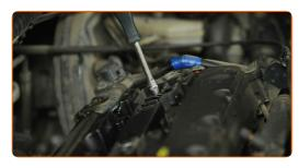
Remove the ignition coil by pulling it straight up.
