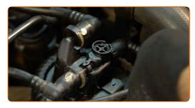
Connect the fuel supply lines to the fuel filter.
