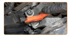
Unscrew the fasteners that connect the engine mount to the car body. Use a drive socket #E14. Use a ratchet wrench.
