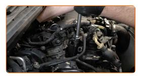
Screw in the fasteners that connect the engine mount to the car body. Use a drive socket #E14. Use a ratchet wrench.
