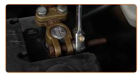
6 Disconnect the earth cable terminal from the battery.
