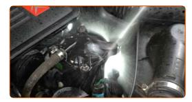
Unscrew the fasteners of the fuel filter cover. Use HEX No.H4. Use a ratchet wrench.
