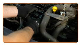
Attach the fuel pressure sensor connector.
