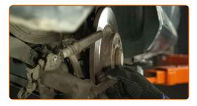
Tighten the brake caliper bracket. Use Torx T55. Use a torque wrench. Tighten it to 108 Nm torque.
