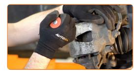
Remove the brake caliper.
