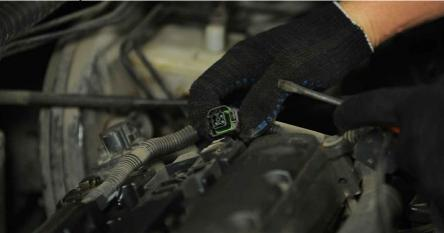
Inscrew the ignition coil bolts. Use a drive socket #8. Use a ratchet wrench.
