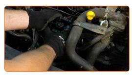
Attach the fuel pressure sensor connector.
