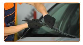
Remove the blade from the wiper arm.
