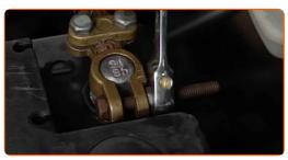
Disconnect the earth cable terminal from the battery.
